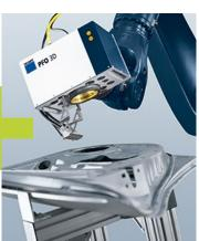
When used with scanner optics, the excellent beam quality of the fiber lasers enables both high processing speeds and large scanning areas.
