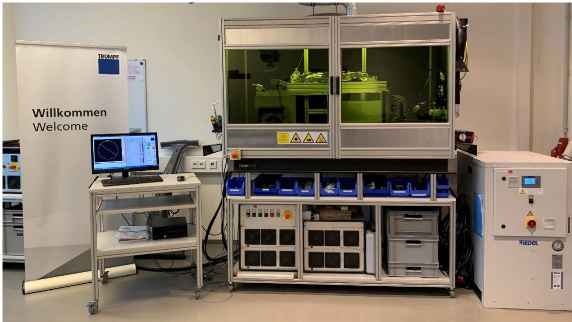
Figure 2: Setup in the Connected Technology Center in Aachen. Laser chamber with cooling unit, driver unit, and control PC
