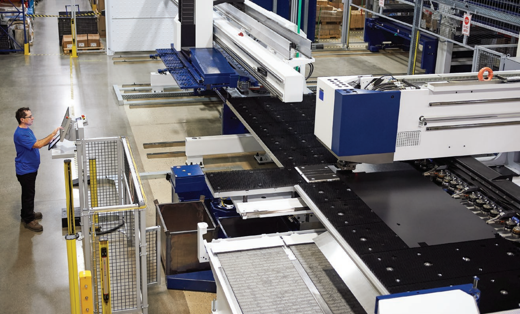
TruPunch 5000: Used for the in-house production of Minus Forty refrigerated merchandisers
